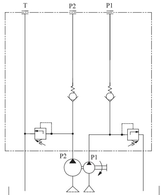
The W85BT series power pack is designed for applications that need two independent hydraulic power supply, but only use a single transmission.
